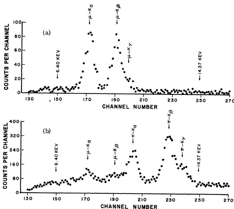
FIG. 2. Pulse-height spectra from Si(Li) detector viewing x rays from (a) muons and (b) pions stopping in He counter. Channel positions corresponding to the calibration energies of  $\text{Co}^{57}$  are indicated by arrows, together with the energies for the Bohr K series in helium.
