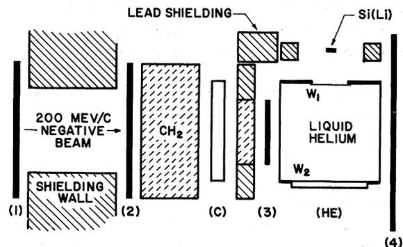
FIG. 1. Plan view of experimental arrangement.  $W_1$  is a 50-mil Be exit window for the x rays.  $W_2$  is a sapphire window through which the scintillation light from the 6-in diameter cylindrical helium counter is viewed. C is a Cherenkov counter used to discriminate against electrons in the beam.
