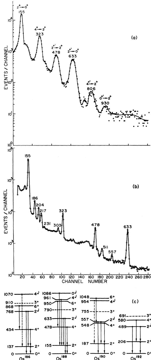
FIG. 1. Gamma-ray spectra for 70.3-MeV  $O^{16}$  ions on  $Os^{188}$ : (a) NaI(Tl) spectrum taken in coincidence with backscattered  $O^{16}$  ions, (b) direct singles spectrum taken with a 7.7-cc Ge(Li) counter, and (c) levels excited in  $Os^{186,188,190,192}$ .
