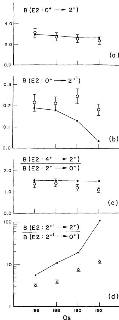
FIG. 2. Comparison of the Kumar and Baranger calculations with the measured reduced transition probabilities for (a) the  $0^+ \rightarrow 2^+$  transitions, and (b) the  $0^+ \rightarrow 2^{+'}$  transitions, and with the ratios (c)  $B(E2:4^+ \rightarrow 2^+)/B(E2:2^+ \rightarrow 0^+)$ , and (d)  $B(E2:2^{+'} \rightarrow 2^+)/B(E2:2^{+'} \rightarrow 0^+)$ . The solid lines join points predicted by the Kumar and Baranger calculations.
