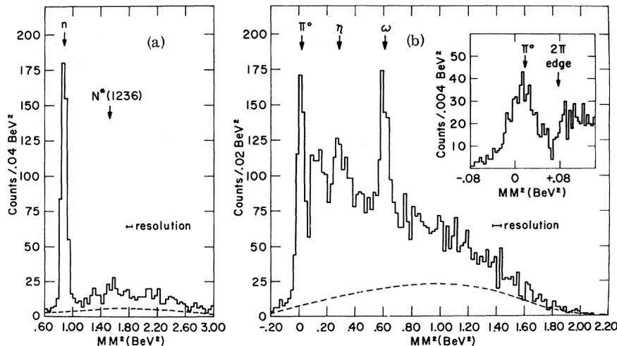
FIG. 3. (a) Total missing-mass square spectrum of events of the type  $p+p \rightarrow p+\pi^++\text{MM}$ . Total number of events is 1234. The dashed line shows the calculated contribution of accidental coincidences ( $311 \pm 44$  events). The horizontal bar indicates the computed resolution. (b) Total missing-mass square spectrum of  $p+p \rightarrow p+p+\text{MM}$ . Total number of events 6331, (calculated accidentals  $1659 \pm 245$ ).
