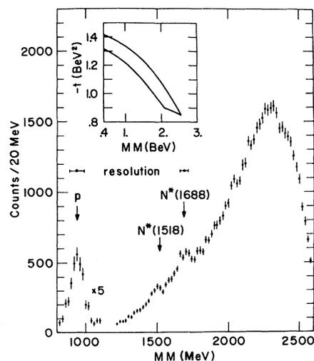
FIG. 2. Missing-mass spectrum for protons detected in the high momentum arm. The total number of events is 55 588. The spectrum shown was obtained at a magnetic field  $B_0 = 15.7 \text{ kG}$  in M1 and M2. The corresponding spectrometer acceptance in the momentum-transfer missing-mass plane for the high-momentum arm is shown in the inset.
