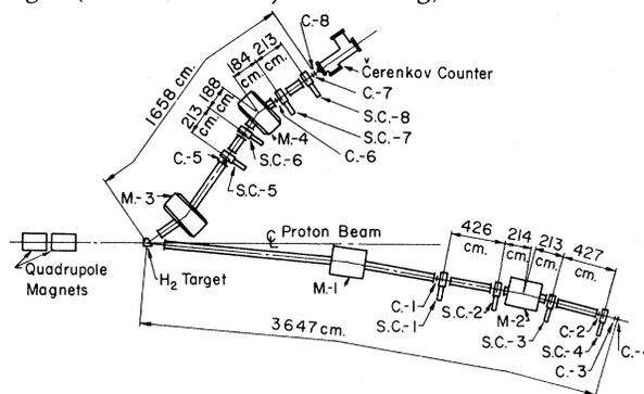
FIG. 1. Experimental layout. C1-C3 and C5-C7 are  $\frac{1}{4}$ -in.-thick scintillation counters for triggering; C4 and C8 are 2-in.-thick scintillation counters for time-of-flight measurement. SC1-SC8 are spark chambers; M1-M4 are bending magnets.
