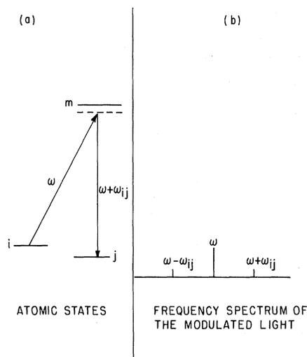
FIG. 1. Double-quantum transitions between two Zeeman levels caused by optical photons.
