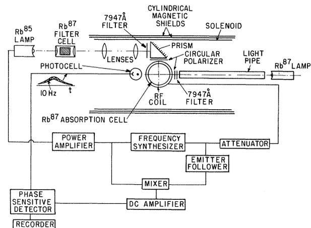
FIG. 2. The spectrometer for coherent detection of optical double-quantum transition.
