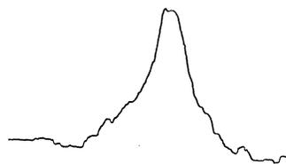
FIG. 3. A recorder trace of an optical double-quantum transition probability versus magnetic field. The integration time was 10 sec.
