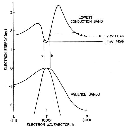
FIG. 2. Schematic of the GaAs band structure near the energy gap showing the relevant excitation-escape processes. For photon energies below 1.7 eV, the electrons thermalize in the  $\Gamma$  minimum before escaping into vacuum, while for larger photon energies, an increasing number "thermalize" in the  $X$  minima.
