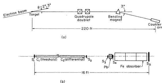
FIG. 1. (a) Beam configuration (not to scale). The target is 0.3 radiation lengths of Be. (b) Counter array (not to scale).  $S_1$ ,  $S_2$ ,  $S_3$ ,  $S_4$ , and  $S_5$  are plastic scintillators;  $C_1$  and  $C_2$  are, respectively, threshold and differential Čerenkov detectors.
