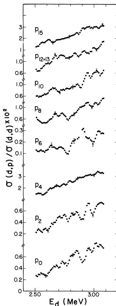
FIG. 2. Three-point running average of the excitation functions for the measured proton groups. The error bars indicate the statistical uncertainty for the three-point sum.
