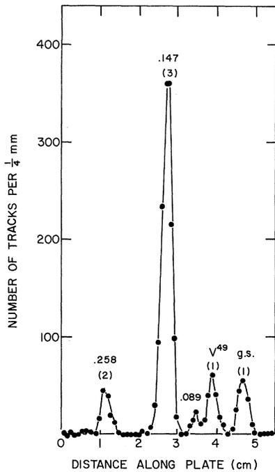
FIG. 1. Deuteron spectrum from the reaction  $\text{Ti}^{46}(\text{He}^3, d)\text{V}^{47}$  measured at  $30^\circ$ . The numbers in parentheses are the values of the orbital angular momenta transferred in the reaction.
