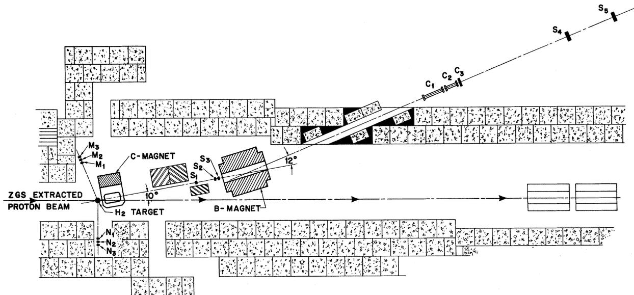
FIG. 1. Layout of experiment. The incident protons come down the extracted beam and strike the hydrogen target. The produced particles are detected by the spectrometer.
