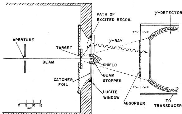
FIG. 1. Experimental arrangement for recoil implantation through vacuum.
