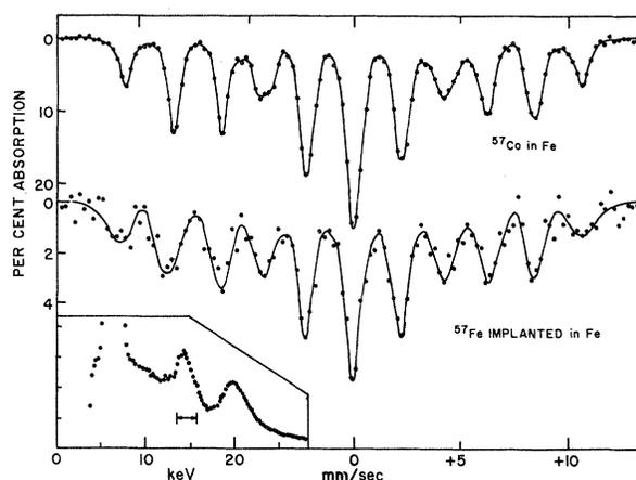
FIG. 3. Mössbauer spectra for excited  $^{57}\text{Fe}$  recoils implanted in Fe metal and for  $^{57}\text{Co}$  diffused into Fe metal. The absorber is an  $^{57}\text{Fe}$  (91%) foil. The broadening of the outermost lines is due chiefly to the "cos $\theta$  effect." The insert shows the gamma-ray spectrum in the implantation measurement; the setting of the 14-keV channel is indicated.
