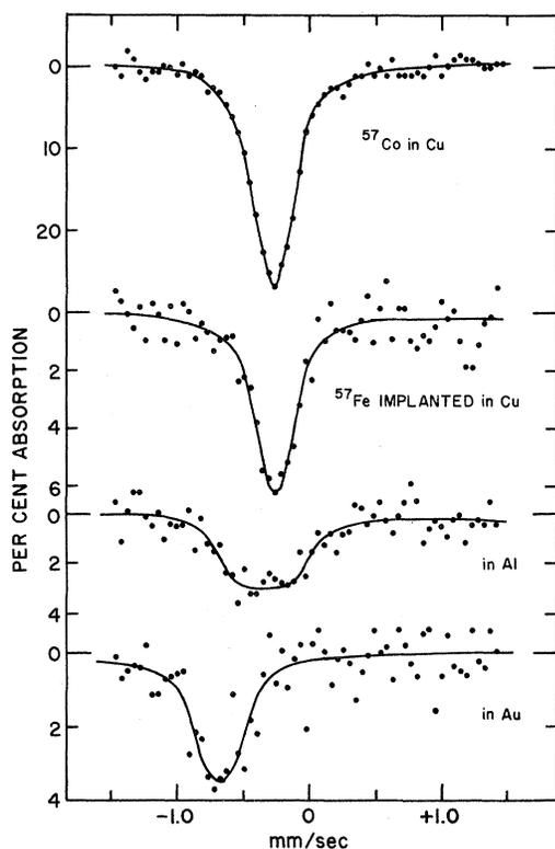
FIG. 2. Mössbauer spectra of excited  $^{57}\text{Fe}$  recoils implanted in different metals, together with a reference spectrum for  $^{57}\text{Co}$  diffused into Cu. The single-line absorber is enriched  $\text{Na}_4\text{Fe}(\text{CN})_6$ . The ordinate is not corrected for background.
