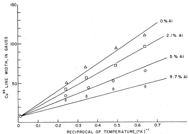
FIG. 1. Low-temperature linewidth of  $\text{Cu}^{63}$  nmr at 8500 G in Cu-Mn alloys containing varying amounts of Al impurities. The Mn concentration is constant at 0.05 at. %.
