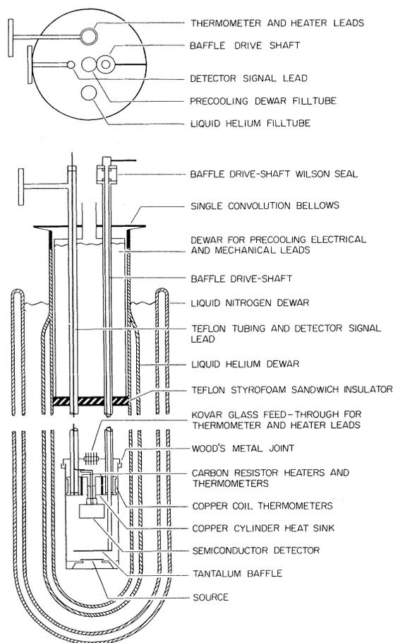
FIG. 1. The cryostat used for the measurement of  $\epsilon$ .
