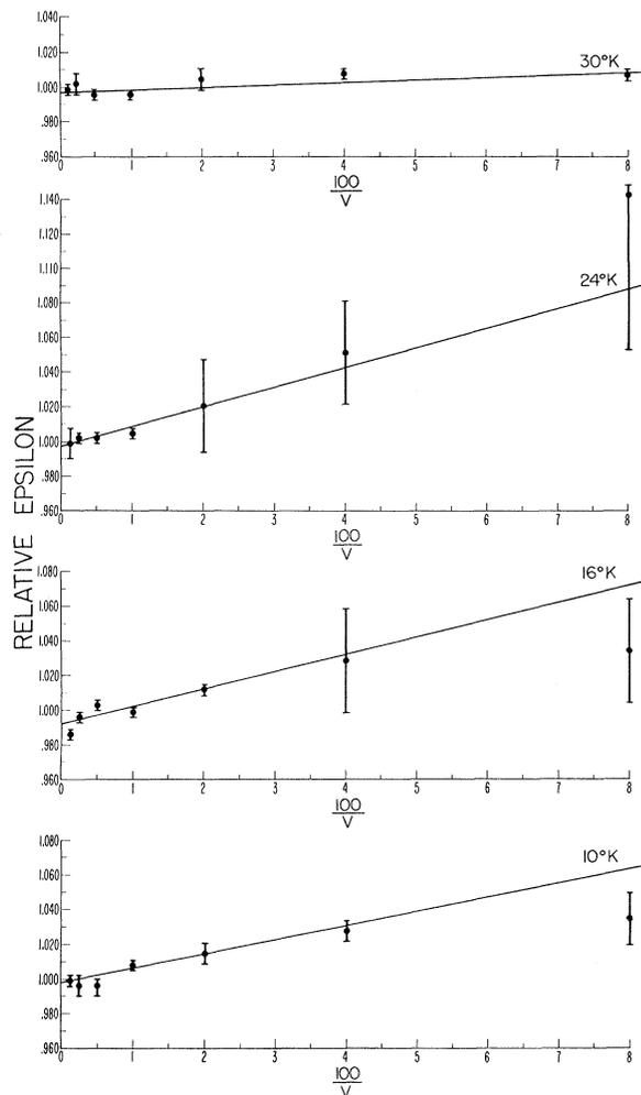
FIG. 2. Relative values of the product  $\eta\epsilon$ , where  $\eta$  is the charge collection efficiency, for 480-keV  $^{207}\text{Bi}$  conversion electrons as a function of the reciprocal of the bias voltage.
