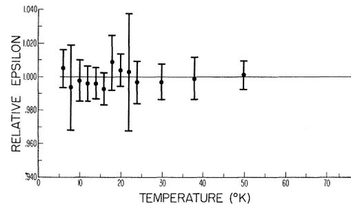
FIG. 3. The mean energy required to create an electron-hole pair normalized to the average value in the temperature interval 6-77°K.
