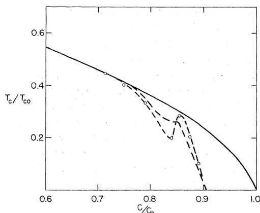
FIG. 1. The dependence of the reduced superconducting transition temperature on the concentration of paramagnetic impurities is shown for the alloy  $\text{La}_{3-x}\text{Gd}_x\text{In}$ . The transition temperature  $T_{c0}$  refers to the superconductor in the absence of paramagnetic impurities. The critical concentration  $c_0 = 2.15$  at.%, the  $s$ - $d$  collision time  $\tau_{\text{ex}}$ , and the solid curve are determined from
