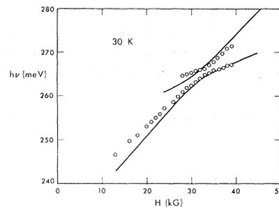
FIG. 3. Field dependence of the infrared absorption in InSb. The solid lines are the theoretical results of Eq. (4). The open circles are the data of Ref. 1.
