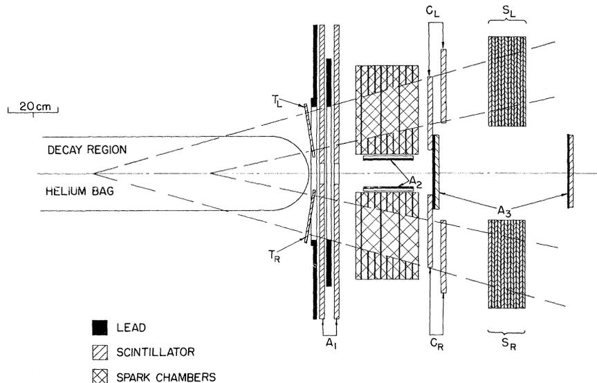
FIG. 1. Geometry of the  $K_2^0 \rightarrow 2\gamma$  experiment (horizontal view).  $A_1$ ,  $A_2$ , and  $A_3$  are lead-loaded anti counters.  $C$  are triggering counters for ionizing particles.  $S$  are shower detectors and  $T$  are counters for the monitoring on the charged  $K_2^0$  decays.
