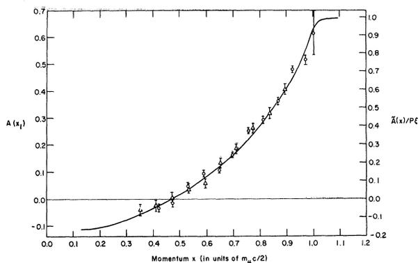
FIG. 3. Experimental decay asymmetry points  $A(x_i)$ , observed (a) with a  $0.42\text{-g/cm}^2$  Li target,  $B = 832$  G (triangles); (b)  $0.40$   $\text{g/cm}^2$  Li,  $B = 1000$  G (circles). The solid line is the best-fit theoretical curve (including corrections)  $\tilde{A}(x; \delta, P)/P\xi$  to all our data (Table I) with  $\delta = 0.758$ . The theoretical curve extends above  $x = 1$  due to finite spectrometer resolution.
