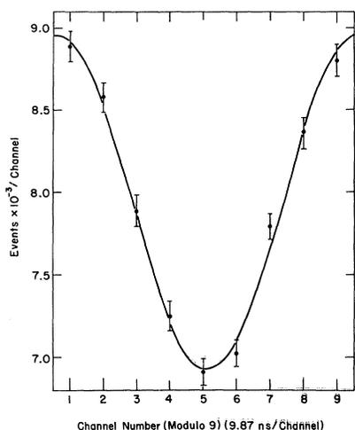
FIG. 2. Over-all ( $0.32 < x < 0.92$ ) precession curve observed with a  $0.42\text{-g/cm}^2$  Li metal target in a field of  $832.0$  G. Data from the first precession period  $T_0$  after  $t = 0$  are discarded, and those from the next 58 are added modulo  $T_0 (= 9$  channels), and corrected for exponential decay. The sine curve fitted to the data has  $\chi^2 = 3.8$  (6 degrees of freedom).
