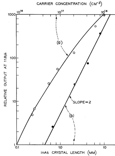
FIG. 2. Total  $11.8$ - $\mu$  output from  $n$ -InAs, (a) as a function of carrier concentration along with the solid line showing the calculated output from Eq. (1) normalized at  $n_e = 10^{16} \text{ cm}^{-3}$ , and (b) as a function of length showing the expected  $l^2$  dependence together with the experimental points.
