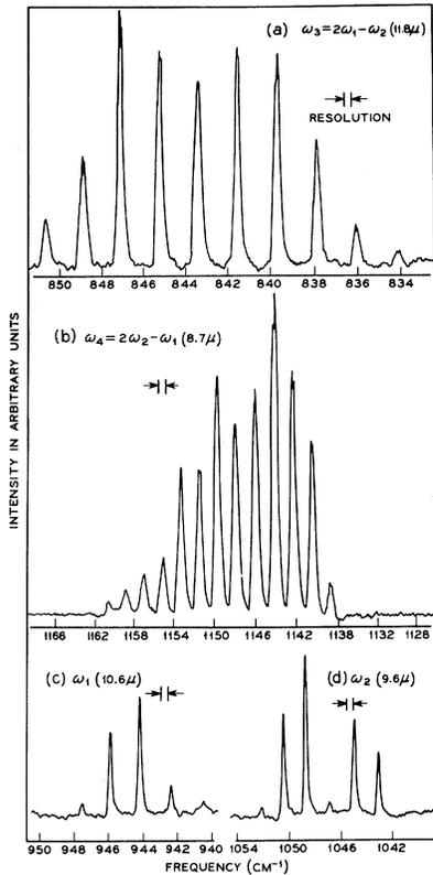
FIG. 1. Output from 1-mm-thick  $n$ -InSb ( $6 \times 10^{16} \text{ cm}^{-3}$ ,  $\sim 80^\circ\text{K}$ ). (a) Mixed signal at  $11.8 \mu$ ; (b) mixed signal at  $8.7 \mu$ ; (c) input signal at  $10.6 \mu$ ; and (d) input signal at  $9.6 \mu$ .
