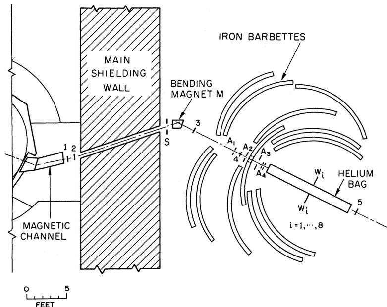
FIG. 1. Layout of the experimental apparatus.
