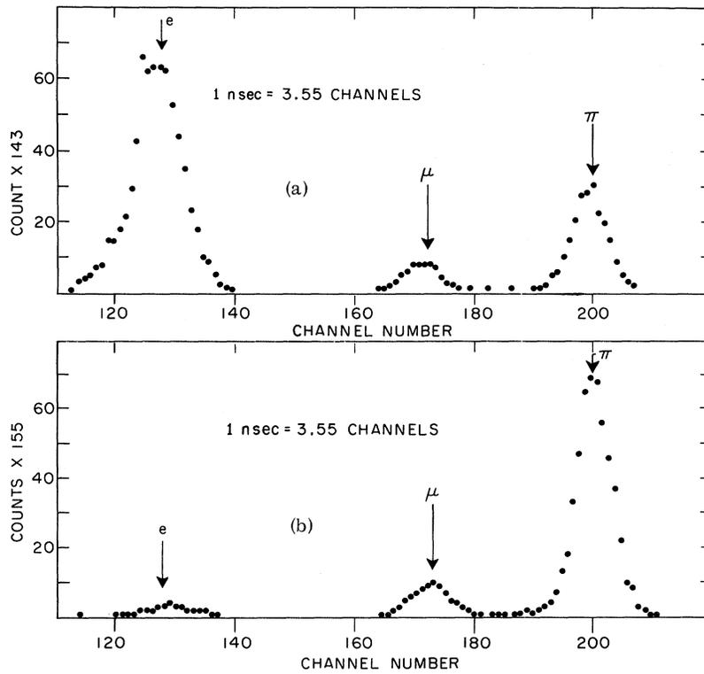
FIG. 3. (a)  $S_2$ - $S_5$  time-of-flight beam spectrum positive. (b)  $S_2$ - $S_5$  time-of-flight beam spectrum negative.
