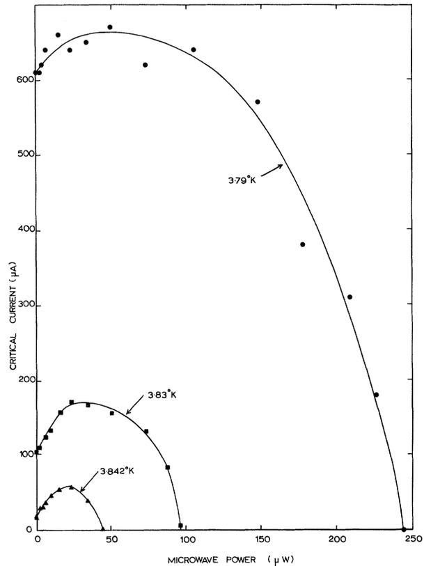
FIG. 1. Critical current through the constriction as a function of microwave power at different temperatures. The "transition" temperature of the film is  $3.845^\circ\text{K}$ .
