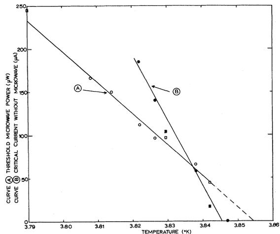
FIG. 2. Curve A shows the threshold microwave power as a function of temperature, and Curve B shows the critical current without microwaves as a function of temperature. Square characters are for the same sample as in Fig. 1. Circular characters are for an identical sample.
