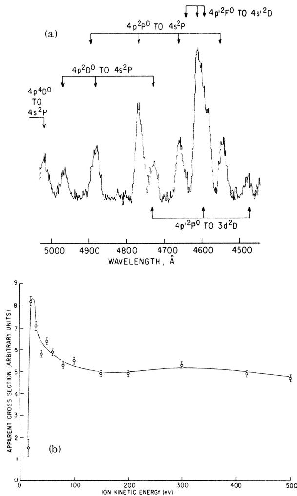
FIG. 2. (a) Spectrum of light emitted in the impact of  $\text{He}^+$  on argon. Wavelength assignments correspond to transitions in the  $\text{Ar}^+$  spectrum. (b) Kinetic-energy dependence of the cross section for the production of  $4764.9\text{\AA}$  line ( $4p^2P^0-4s^2P$ ) by  $\text{He}^+$  impact on Ar.
