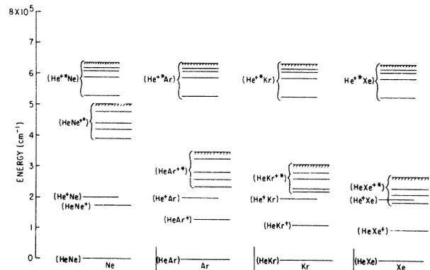
FIG. 3. Relevant energy levels for separated ( $R \rightarrow \infty$ ) rare-gas molecular systems.
