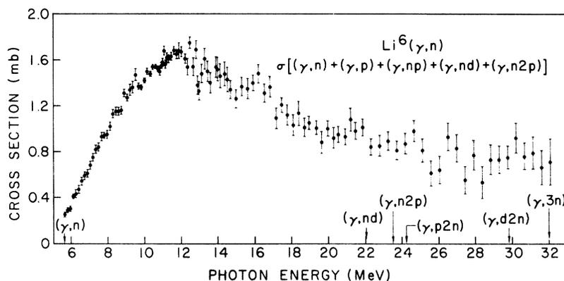
FIG. 1.  $\text{Li}^6$  single-neutron-production cross section. This contains all partial cross sections except (a) those where all the emitted particles are charged, and (b) those where two or more neutrons are emitted. The errors given are statistical only.
