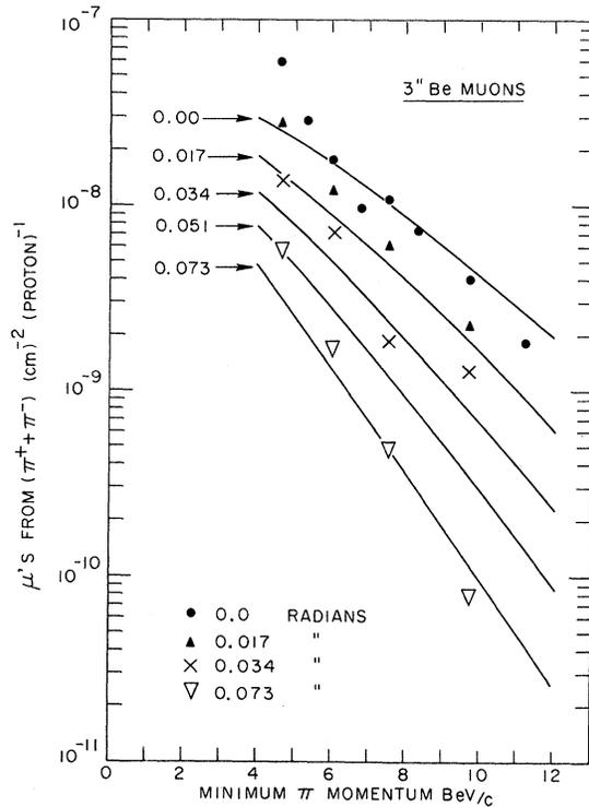
FIG. 3. Emulsion data compared to the muon spectra calculated from beam survey data for 30-BeV/ $c$  protons. The data shown are normalized on a plane 100 ft from a 3-in. Be target.
