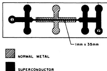
FIG. 1. Geometry of tunneling junction. Tunneling measurements are made between the normal metal and the superconductor while a transport current is passed between terminals 1 and 2.
