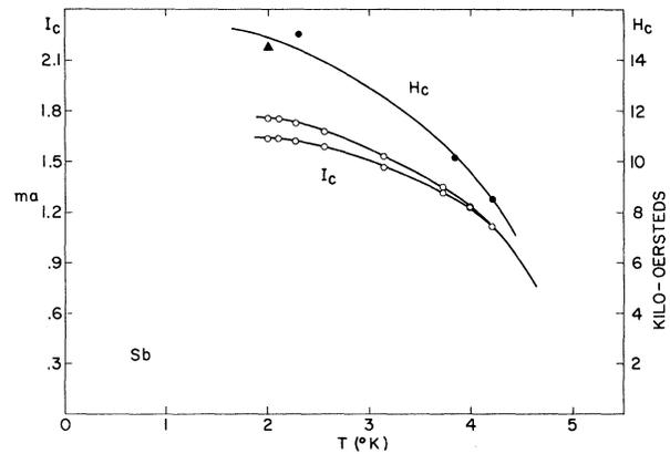
FIG. 2.  $I_C$  and  $I_C'$  (open circles) with  $H=0$ , vs  $T$ , and  $H_C$  vs  $T$  (closed circles) for one Al on Sb sample. One point (triangle) of  $H_C$  vs  $I$  for another Al on Sb sample.
