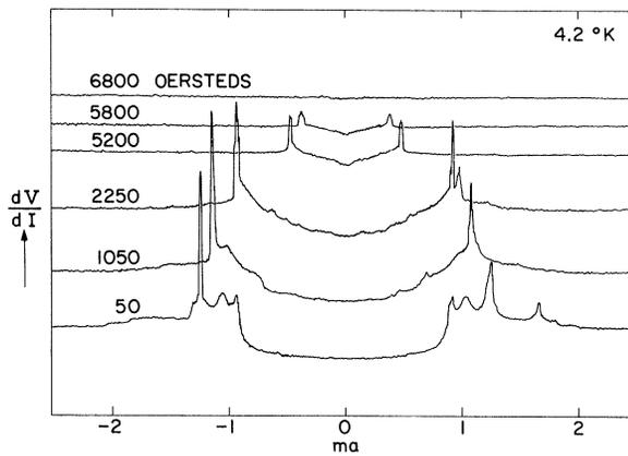
FIG. 3. A plot of  $dV/dI$  vs  $I$  for Al on Sb for different magnetic fields. The zero level of  $dV/dI$  was shifted for each curve.
