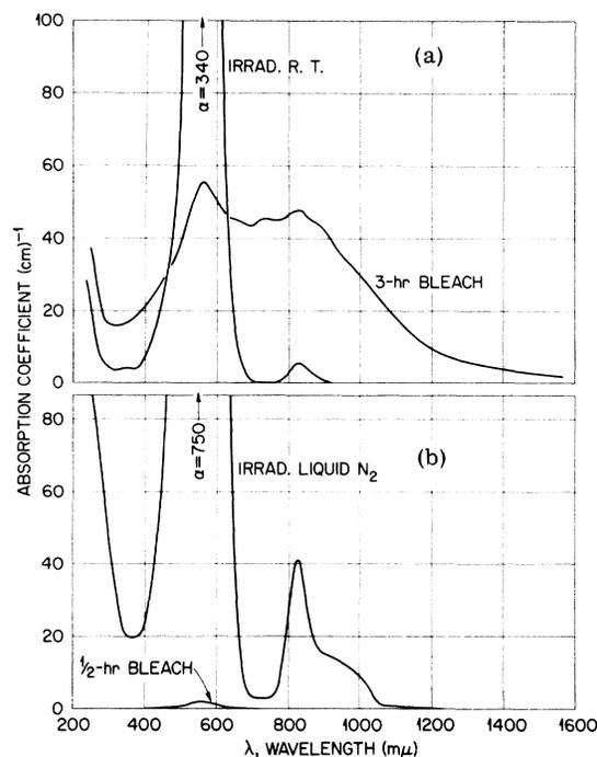
FIG. 1. Room-temperature spectra of KCl crystals. (a) Irradiation at room temperature; (b) irradiation at 80°K. In each case the spectrum with the large *F* band at 560  $\text{m}\mu$  was obtained before bleaching and the other spectrum was obtained after bleaching with white light.
