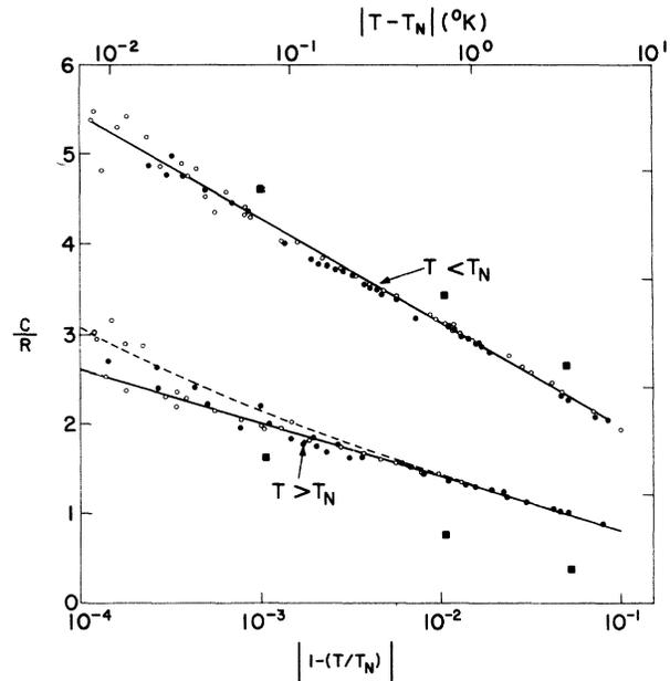
FIG. 1. Magnetic specific heat of  $\text{MnF}_2$  near the Néel temperature. Open circles, IBM crystal; closed circles, Heller and Benedek crystal. The closed squares are the specific-heat density of argon. The dashed curve is for  $\alpha = 0.1$ .
