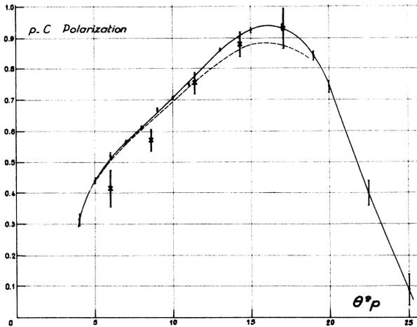
FIG. 3. Proton-carbon polarization at 220 MeV. Solid points: data of reference 3; crossed points: our results. The dashed line is the polarization calculated when taking into account some inelastic proton-carbon scattering.
