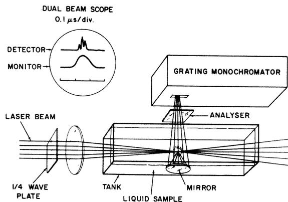
FIG. 1. Arrangement for observation of nonlinear scattering. The polarization properties of the scattered light were determined with the laser both plane and circularly polarized. The signal from a 1P28 phototube which measured the scattered radiation through the monochromator, along with that from a monitor of the laser beam, was displayed on a dual-beam oscilloscope. Individual photoelectrons could be detected. Spurious signals occurred during the laser pulse about once in every 200 pulses.
