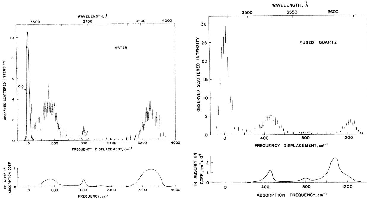
FIG. 2. Observed unpolarized nonlinear scattering spectra and infrared absorption spectra for water and fused quartz. The scattering intensity is given in photoelectrons per laser pulse (½-MW peak power in the case of water, 1-MW for fused quartz) averaged over approximately 25 pulses. Standard errors are indicated. When no signal was observed, the 70% probability limits using Poisson statistics are shown. The spectrometer band pass was 80 cm<sup>-1</sup>.
