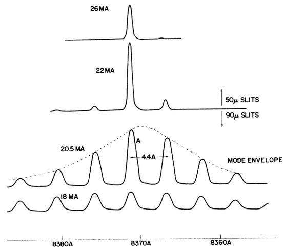
FIG. 1. Mode structure of the laser in the region of threshold. The intensity (vertical scale) is different at each current. The mode envelope at 20.5 mA is indicated by the dashed line. In all cases the widths of the peaks are instrument limited.
