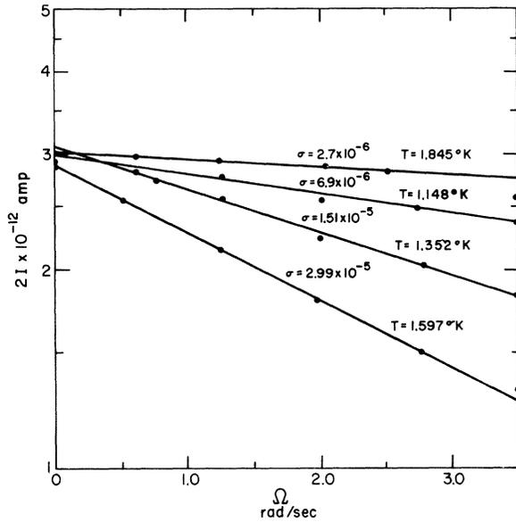
FIG. 2. Current  $I$  as a function of angular velocity  $\Omega$ , measured by the cell shown in Fig. 1. The voltage  $V$  between  $G$  and  $C_1$  is 200 V. The solid lines represent Eq. (1) for the cross sections shown.
