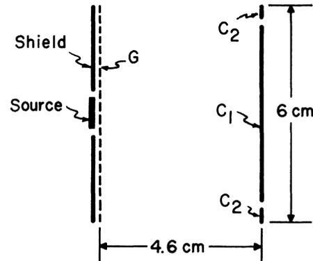
FIG. 1. Cell used to measure cross sections. The source measures 1 cm by 0.3 cm; the shield, grid  $G$ , and guard  $C_2$  measure 6 cm by 3.5 cm.
