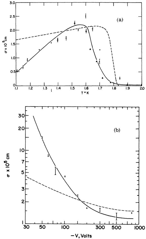
FIG. 3. (a) Cross section as a function of temperature for  $V = 200$  V. The solid circle and solid triangle refer to measurements made at widely separated times. (b) Cross section as a function of  $V$  at a temperature of 1.46°K. The continuous curves indicate only the experimental relationships. The dashed curves represent the theoretical cross sections corrected according to Eq. (2).
