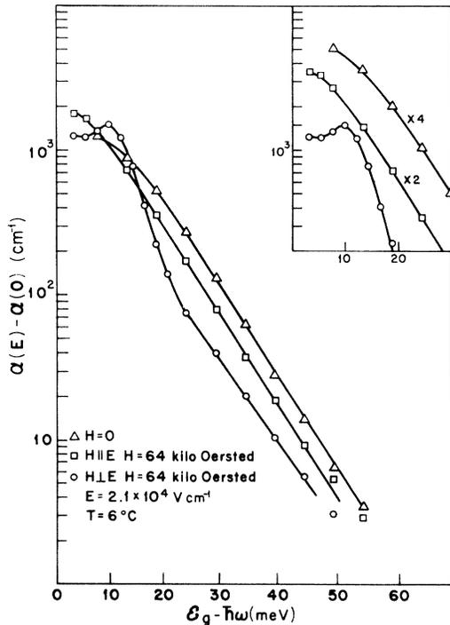
FIG. 1. Electric-field-induced optical absorption below the direct gap in germanium at 6°C, for  $E = 2.1 \times 10^4$  V/cm,  $H = 0$ , and  $H = 64$  kOe in the longitudinal and transverse configuration. In crossed fields a resonance shows up approximately 10 meV below the gap. In the inset the absorption curves for  $H||E$  and  $H = 0$  have been multiplied by factors of 2 and 4, respectively, to show the resonance more clearly.
