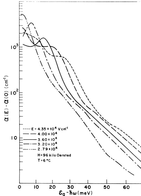
FIG. 2. Electric-field-induced optical absorption below the direct gap in germanium at 6°C, for  $H \perp E$ ,  $H = 96$  kOe, and for various values of *E*. With increasing *E* the resonance shifts to lower photon energies and decreases in intensity.
