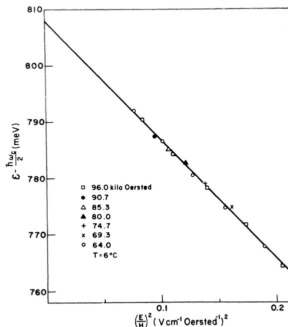
FIG. 3.  $\epsilon$ , the energy at which the resonance occurs, diminished by  $\hbar\omega_c/2$ , the sum of the magnetic energy of the zeroth Landau levels in the conduction and valence band, as a function of  $(E/H)^2$ .
