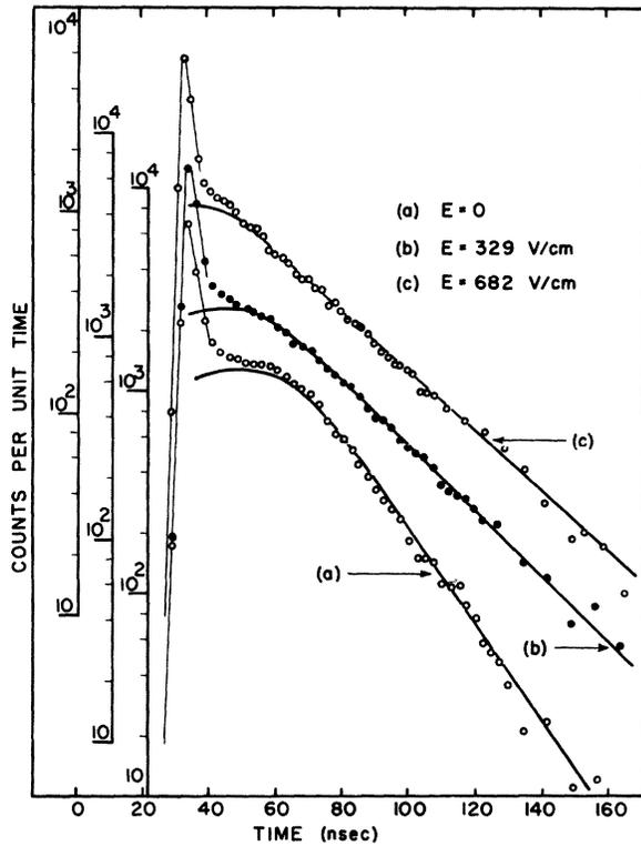
FIG. 2. Direct positron-annihilation spectra in argon for several values of applied electric field. Both the random coincidence background and the ortho-positronium component have been subtracted. The argon pressure was 10.5 atm at 25°C. Lifetimes of each of the exponential decays are (a)  $17.9 \pm 0.7$  nsec, (b)  $26.9 \pm 1.0$  nsec, and (c)  $34.8 \pm 1.5$  nsec.
