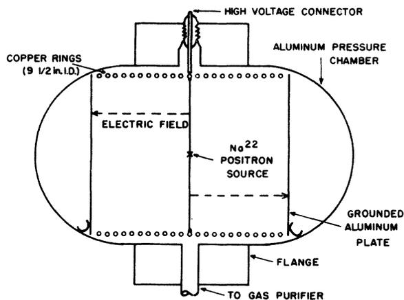
FIG. 1. Gas pressure chamber with field-defining electrodes.
