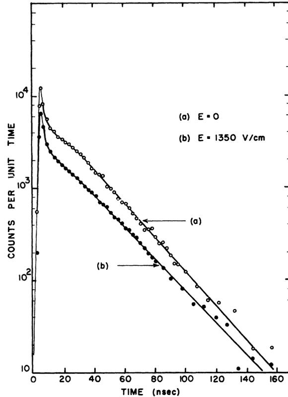
FIG. 3. Direct positron-annihilation spectra in helium with and without an applied electric field. Both the random coincidence background and the ortho-positronium component have been subtracted. The helium pressure was 59.7 atm at 25°C. Lifetimes of each of the exponential decays are (a)  $9.6 \pm 0.5$  nsec, and (b)  $10.3 \pm 0.5$  nsec.
