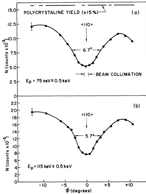
FIG. 1. Copper *L* x-ray yield at 75 and 115 keV. Typical experimental conditions are as follows: proton current  $\approx 0.1 \mu\text{A}$ ; integrated current =  $5 \mu\text{C}$ ; detector background  $\approx 200$  counts. The polycrystalline yield (same for polycrystalline target and 600-grit sanded single crystal) was found to be independent of angle over the range studied. Under the present conditions the effect of x-ray absorption can be neglected.
