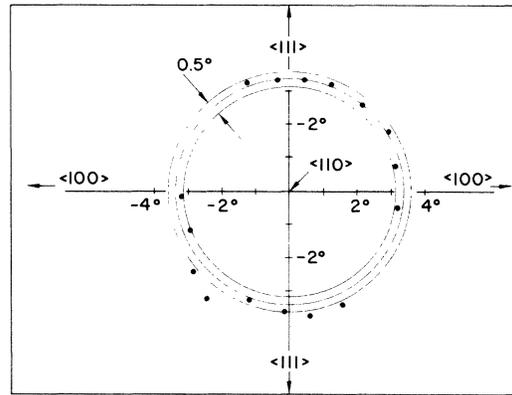
FIG. 2. Angular symmetry of half-width points. The half-width points (8000 counts) for 75-keV proton bombardment of copper show symmetry about the  $\langle 110 \rangle$  direction.
