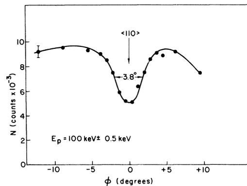
FIG. 3. Aluminum *K* x-ray yield at 100 keV. Experimental conditions are the same as described in Fig. 1.
