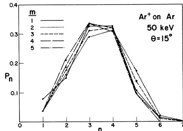
FIG. 1. Charge-state correlation diagram for Ar<sup>+</sup>-on-Ar collisions at 50 keV,  $\theta = 15^\circ$ .
