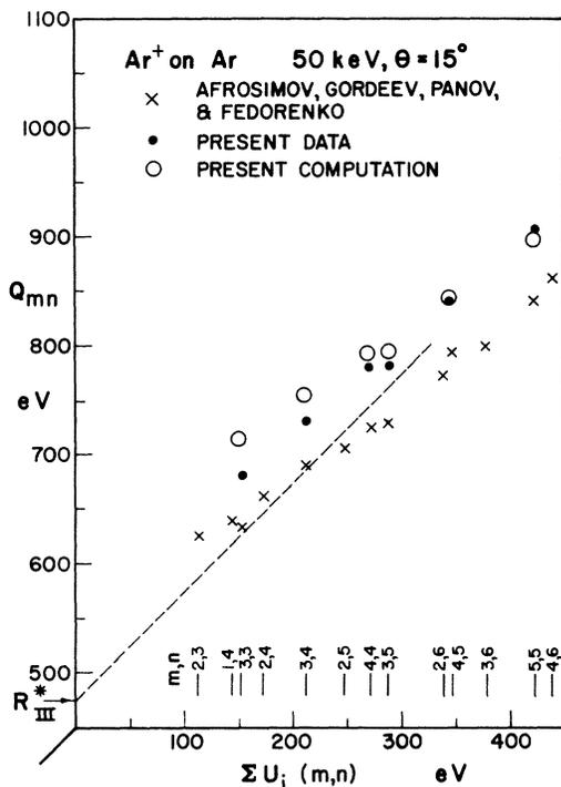
FIG. 2. Inelastic energy loss is plotted versus the net ionization energies for  $\text{Ar}^+$ -on- $\text{Ar}$  collisions where in the charge states  $m, n$  of both particles after the collision are specified. The dashed line is fitted to the data of Afrosimov et al.<sup>1</sup> using Eq. (2). The open circles correspond to the present data and are computed herein.
