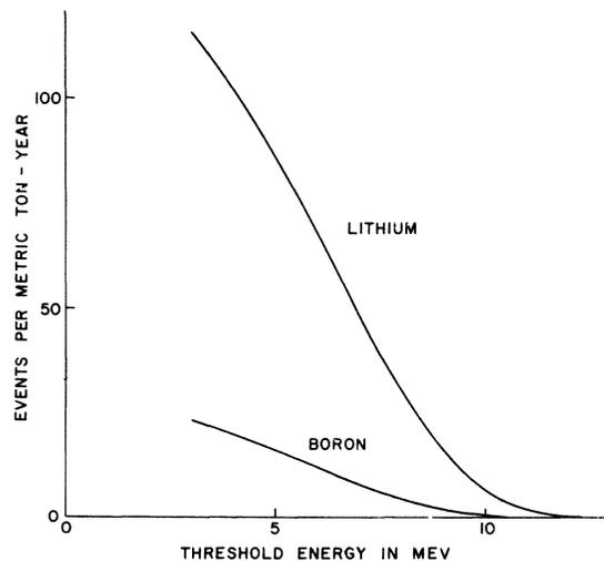
FIG. 2. Count rate for flat slab (2.5 cm Li, 0.5 cm B) vs threshold energy for product electron.
