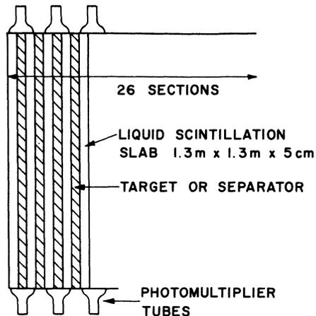
FIG. 5. Schematic of detector. The target or separator sheets will be coated white and wrapped in thin plastic, the latter to produce total internal reflection of the scintillation light.
