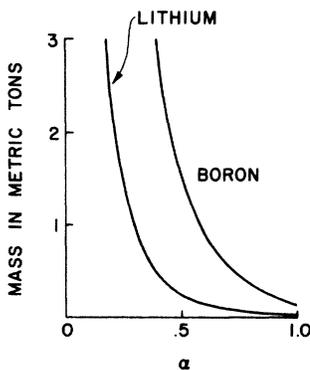
FIG. 4. Target mass needed to detect direction of the sun.
