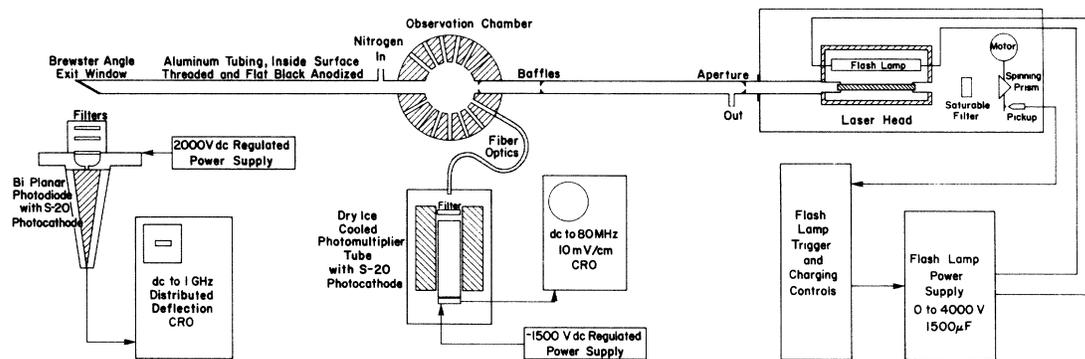
FIG. 1. Diagram of experimental arrangement for the measurement of Rayleigh scattering.
