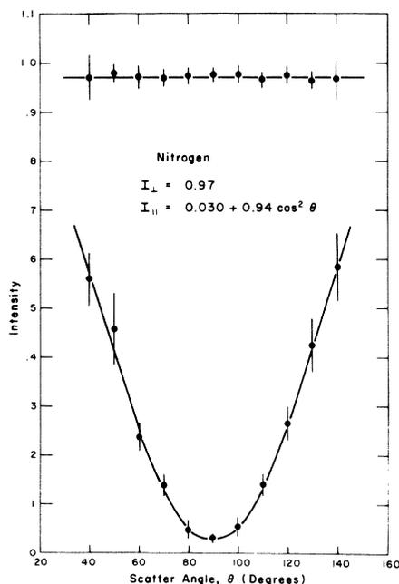
FIG. 2. Angular distribution of scattered radiation in nitrogen at atmospheric pressure and temperature for perpendicular- and parallel-polarized incident light.
