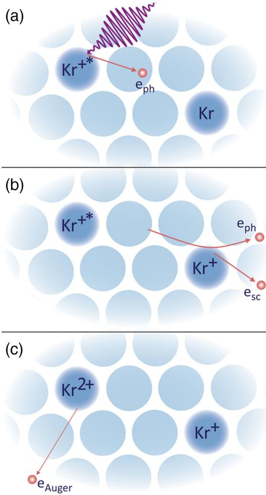
FIG. 1. Sketch of the process under investigation. (a) A Kr atom in a cluster is photoionized in the  $3d$  orbital. (b) On its way through the cluster, the photoelectron scatters inelastically at another atom and ionizes it. (c) The initially ionized atom decays by Auger electron emission.
