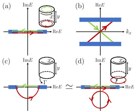
FIG. 2. (a),(b) Chern insulator under the periodic boundary condition in the  $x$  direction and the open boundary condition in the  $y$  direction. A chiral edge mode (red) at the bottom boundary and an antichiral edge mode (green) at the top boundary form a loop on the real axis in the complex energy plane. (c) Chern insulator (a) with the decay constant term  $\Gamma$  at the bottom boundary. (d) Chern insulator (a) attached the Hatano-Nelson model at the bottom boundary.
