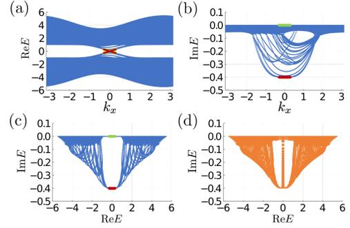
FIG. 4. 3D chiral symmetric topological insulator ( $L_x = 300$ ,  $L_y = L_z = 20$ ) in Eq. (5) with  $-i\Gamma\sigma_0\tau_0$  ( $\Gamma = 0.2$ ) term at the  $z = 1$  boundary. (a)–(c) The real and imaginary parts of the spectrum under the periodic boundary conditions in the  $x$  and  $y$  directions. (d) The complex spectrum under the periodic boundary condition in the  $x$  direction and the open boundary condition in the  $y$  direction. There appear in-gap boundary modes.
