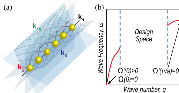
FIG. 1. (a) An infinite chain of identical masses. Each mass is connected to its  $n$ th-nearest neighbors with spring constant  $k_n$ . (b) The design space with fundamental constraints at the center ( $q = 0$ ) and edge ( $q = \pi/a$ ) of the first Brillouin zone.
