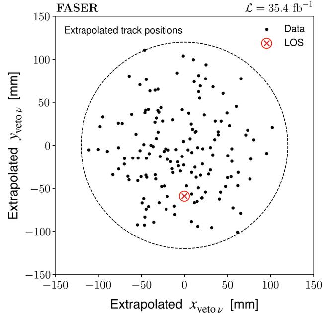
FIG. 3. Extrapolated transverse position of the reconstructed tracks of neutrino-like events to the FASER $\nu$  scintillator station. The ATLAS LOS is indicated with a red marker and shifted 59 mm in the negative  $y$  direction from the center of the scintillator station.
