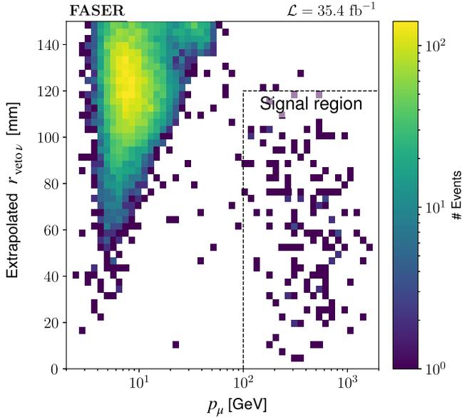
FIG. 2. The selected signal region in extrapolated radius  $r_{\text{veto}\nu}$  and reconstructed track momentum  $p_{\mu}$  is depicted. The region with lower momenta and larger radii is dominated by background events consisting of charged particles that miss the FASER $\nu$  scintillator station.
