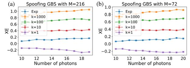
FIG. 3. (a) 216 modes with 216 squeezed states with  $r \approx 0.89$ . (b) 72 modes with 72 squeezed states with  $r \approx 0.53$ . The error bar represents the standard deviation of  $\log p_U(x)$  of obtained samples divided by  $\sqrt{N_s}$ , and  $N_s = 10^3$ .
