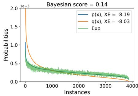
FIG. 5. Bayesian test using  $M = 16$  and  $N = 4$  case in Ref. [12]. The green curve is the experimental data from Ref. [12]. The XE score is different from Fig. 2 because the probability is normalized over the sector for this figure.
