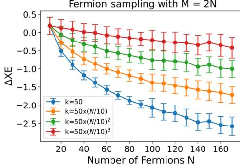
FIG. 4. XE of FS.  $N_s = 10^3$  for  $N \leq 90$  and  $N_s = 10^2$  for  $N \geq 10^2$ . We used  $10^3$  different random unitary matrices for circuit configuration. The error bar represents the standard deviation of XE difference.
