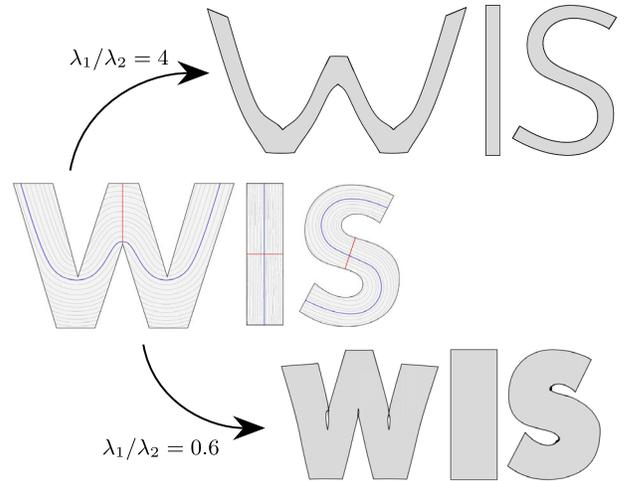
FIG. 4. A PLCE designed to change the font weight of a text. The initial  $u$  curves are chosen to run along the letters' backbones, while the  $v$  curves are chosen to be straight lines. Actuation makes the font either lighter ( $\lambda_2 < \lambda_1$ ) or bolder ( $\lambda_1 < \lambda_2$ ), without buckling out of the plane.
