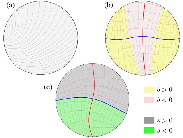
FIG. 3. Geodesic curvature changes of the director field integral curves. (a) the nematic director is everywhere positively bent and positively splayed. The geodesic curvatures of both sets of integral curves are everywhere nonzero. (b) here, the bend  $b$  changes sign twice while  $s$  remains positive; the change of signs occurs along  $v$  curves, a hallmark of LPCEs. (c) similarly,  $s$  could only change sign across  $u$  curves.
