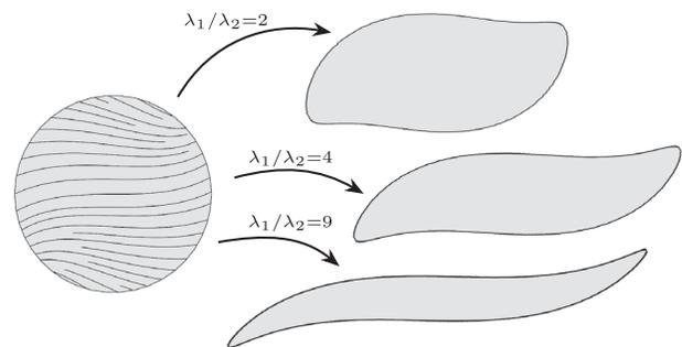
FIG. 1. Planar liquid crystal elastomer (PLCE) deformations of a circular domain. The elongations along (by factor  $\lambda_1$ ) and perpendicular ( $\lambda_2$ ) to the director field deform the sheet and change the shape of its boundary, without buckling out of the plane (regardless of the sheet's thickness).
