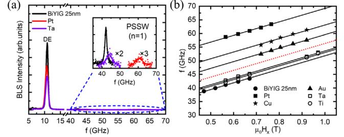
FIG. 3. (a) Exemplary BLS spectra of bare 25 nm BiYIG and BiYIG covered with Pt and Ta. Inset is enlarged PSSW modes, magnified 2 and 3 times its intensity for Pt and Ta overlayers, respectively. (b) The frequency of measured PSSW modes as a function of  $\mu_0 H_x$  with  $q_{\parallel} = 0$ . The expected frequency with measured  $A$  and  $K_s$  with Pt overlayer is plotted with a dotted red line.
