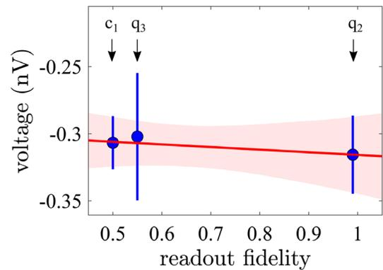
FIG. 3. Detected open-switch voltage as a function of readout fidelity. Mean voltages obtained for each of the bit strings  $c_1$ ,  $q_2$ ,  $q_3$  are marked with arrows. Each error bar corresponds to Gaussian standard error of the mean. The red line shows the best linear fit, and the shaded region indicates the 1-standard-deviation uncertainties in the linear fit parameters, obtained using a Monte Carlo simulation with  $10^4$  realizations.
