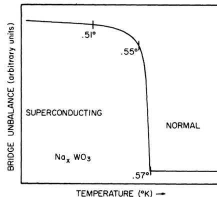
FIG. 1. Superconductivity of sodium tungsten bronze as read directly on an X-Y recorder.
