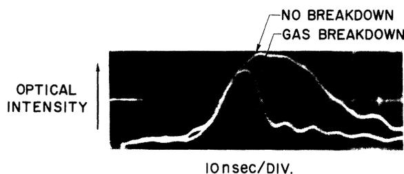
FIG. 2. Attenuation of laser beam by breakdown plasma.
