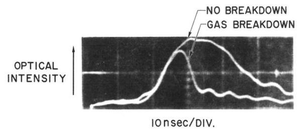
FIG. 2. Attenuation of laser beam by breakdown plasma.
