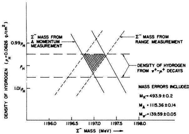
FIG. 4.  $\Sigma^-$  mass from range, momentum, and density of hydrogen measurements, as explained in the text.
