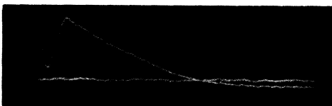
FIG. 1. Time-resolved synchrotron radiation at 1-mm wavelength; sweep speed is 0.5 millisecond per division.
