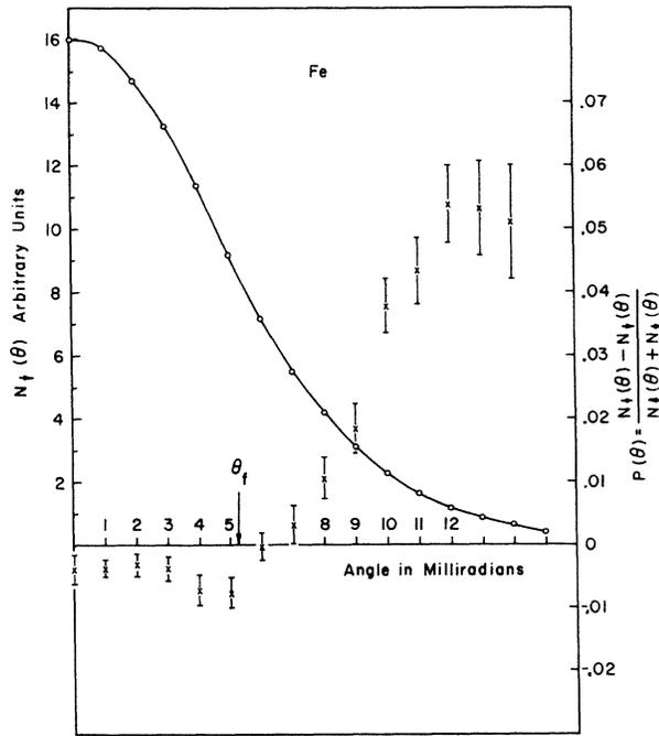
FIG. 1.  $N_{\downarrow}(\theta)$  (left-hand scale) and  $p(\theta)$  (right-hand scale) for polycrystalline iron. The statistical errors for  $N_{\downarrow}(\theta)$  are smaller than the circles. The angular resolution is 0.75 mrad. Arrow indicates the angle  $\theta_F$  corresponding to the free Fermi momentum based on one electron per atom in the conduction band.
