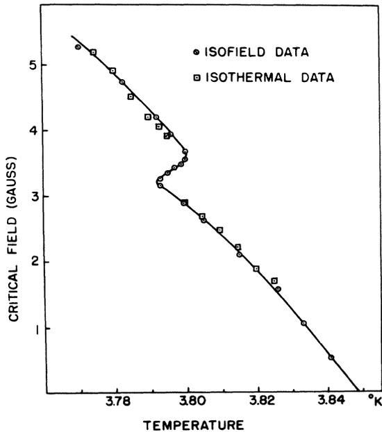
FIG. 4. Critical field vs temperature curve for a tin bridge  $2.65 \mu$  wide, obtained from both isothermal and isofield measurements.
