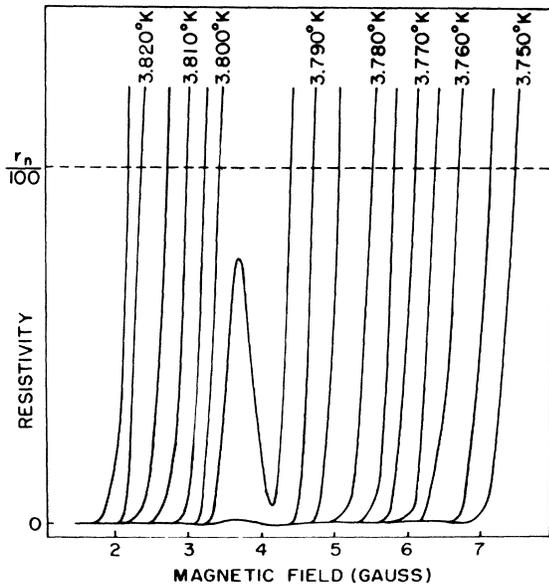
FIG. 2.  $x$ - $y$  recorder tracings of the isothermal resistive transition curves for a tin bridge 2.65  $\mu$  wide.
