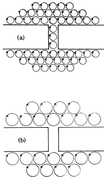
FIG. 3. (a) Vortex configuration in region of microbridge for a perpendicular magnetic field of magnitude  $H_b = \phi_0/\pi R_b^2$ , where  $2R_b$  is the width of the microbridge. (b) Vortex configuration for a field smaller than  $H_b$ .
