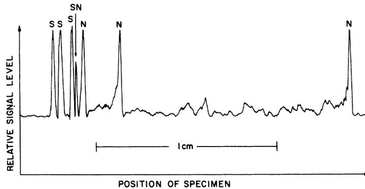
FIG. 2. Interferometer signal level as a function of wire position. Signal level is periodic in the enclosed flux with a period  $h/2e$ . Constant null position and the observed  $2\pi$  phase shift associated with the signal peaks can only be explained by flux pinning in quantum units  $h/2e$ . S and N indicate the direction of the emerging field.
