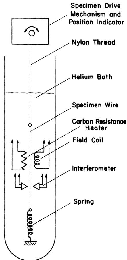
FIG. 1. Schematic representation of the experimental apparatus. This apparatus is shielded by a combination of Mumetal and superconducting shields. The specimen wire is slowly drawn vertically through the interferometer causing discrete phase shifts due to flux leakage.
