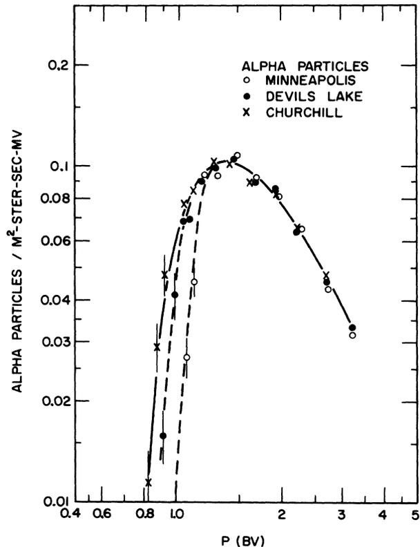
FIG. 3. Differential intensities of primary alpha particles observed at three locations.  $P$  is the particle rigidity defined as momentum/unit charge and expressed in units of BV.
