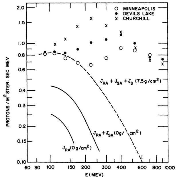
FIG. 1. Proton intensities at a depth 7.5 g/cm<sup>2</sup> at three locations. Intensities of secondary protons and splash and re-entrant albedo are also shown as a function of the particle kinetic energy in MeV.
