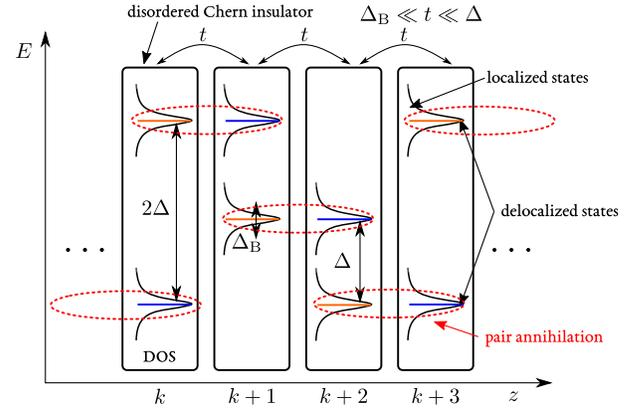
FIG. 4. Sketch of the layer construction for the three-dimensional TLI. A stack along  $z$  direction of two-band disordered Chern insulators, with the bandwidth  $\Delta_B$  and the gap  $\Delta$  or  $2\Delta$ , becomes fully localized due to interlayer coupling  $t$  such that  $\Delta_B \ll t \ll \Delta$ . For each layer, density of states (DOS) is shown, and the delocalized states depicted in orange (blue) carry a positive (negative) quantized Hall conductance.
